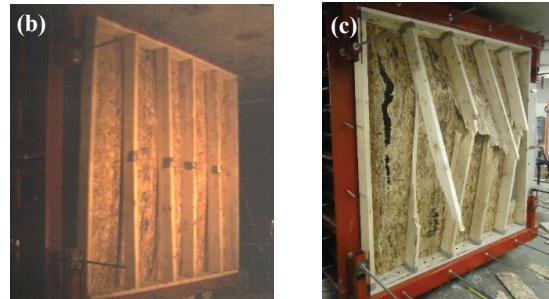
Figure 7: a) PI Diagram for Light-Frame Wood Stud Walls, b) Failure of Nailed Connections, and c) Oversized Connections
