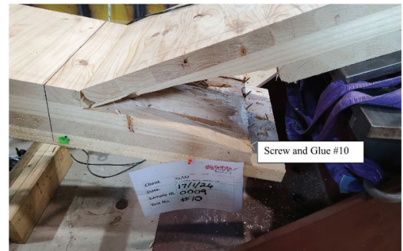
Figure 5 – Typical failure modes: Control samples (top centre), Type A screw only (bottom left) and Type B screw + glue (bottom right)
