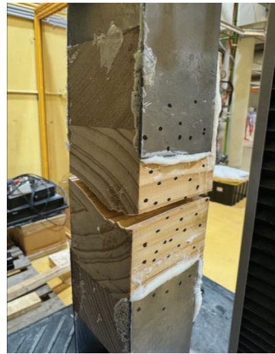
Figure 10. Steel Adhered Perpendicular to Grain Failure Mode
