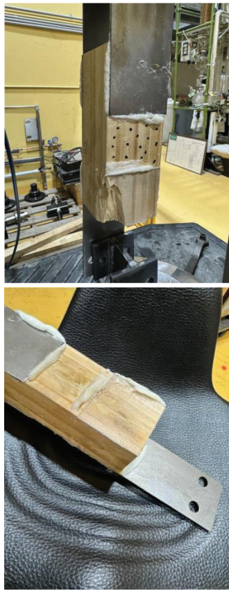
Figure 9. Steel Adhered Parallel to Grain Failure Mode, Glulam 4 (top) and all other samples (bottom)
