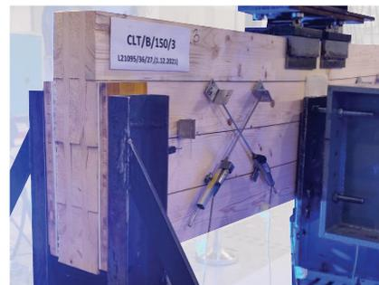
Figure 1. Experimental test setup for prismatic CLT beams (left) and an example of a CLT beam during testing (right).
