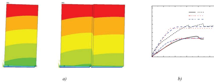
Figure 5. a) Deformation diagram of finite element model, b) Comparison of model and monotonic test result
