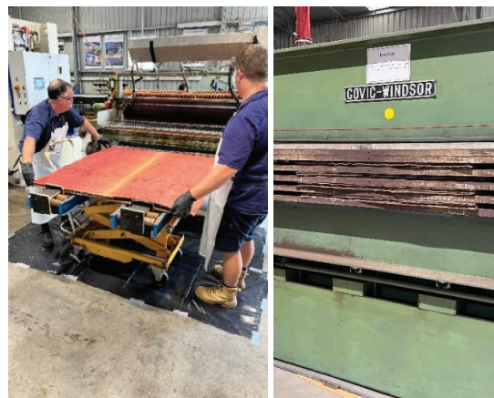
Figure 4. Selected stages of the LVL manufacturing (a) applying adhesive with a double roller glue spreader and (b) LVL being hot-pressed.
