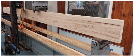
Figure 5. GLT beam tested in four-point bending.
