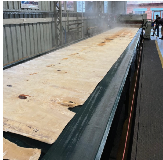
Figure 2. Veneer ribbon obtained after peeling.
