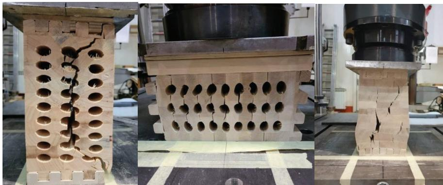
Figure 10 Failure modes
