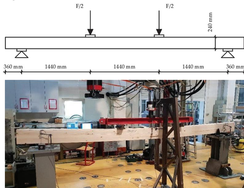
Figure 4. Four-point bending test setup.
