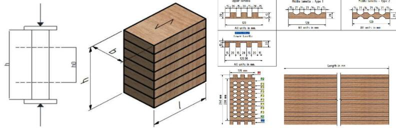
Figure 5. Load and gauge position, specimen dimensions.
