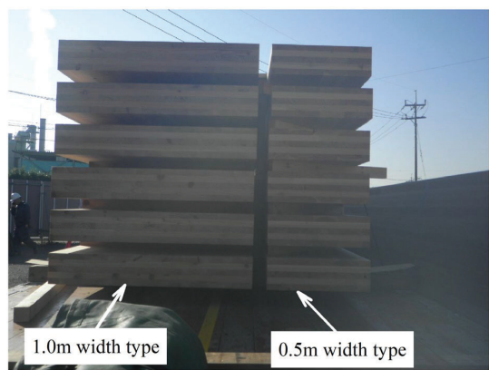
Figure 3. Full-scale CLT used for the experiment
