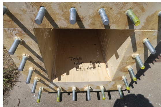
Figure 17: Failure mechanism four point bending test
