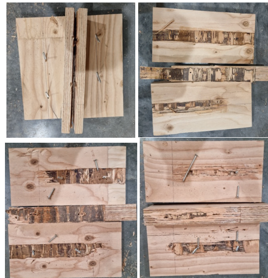
Figure 9. Failure mode of screw-only group, glue-only group and screw-glue groups
