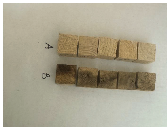
Figure 2. hinoki blocks from Kyushu before (A) and after (B) exposure to R. placenta .
