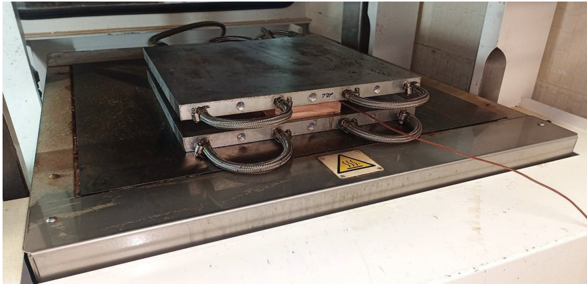
Figure 1. The employed hot press including removable cooling platens and the thermocouple for measuring board temperature. .
