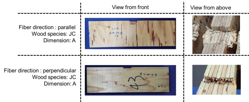
Figure 20. Comparison of fractures loaded parallel and perpendicular to the grain.
