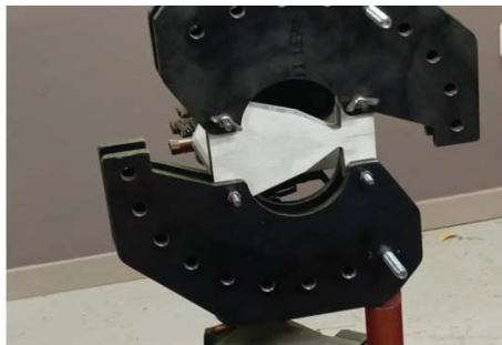
Figure 6 : Setting up the MMCG specimen
