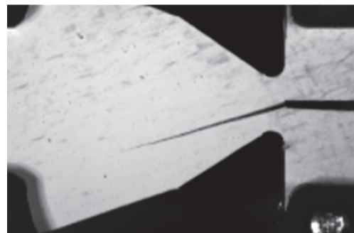
Figure 8 : Specimen M23-a, after the crack at t = 700s
