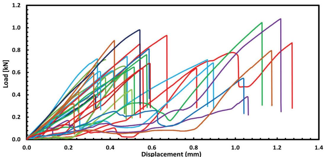
Figure 3. Load-displacement curves of the NWC tests, immediately tested (day 0) under the DRY condition. Most of the nails immediately engaged in linear-elastic-like behaviour (peak on the left side), whereas some nails exhibited significant slip before engagement (peaks on the right side).
