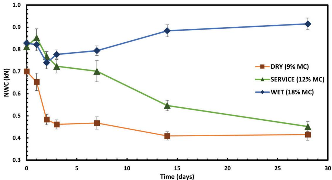
Figure 4. Changes in average NWC on radiata pine conditioned at DRY, SERVICE, and WET conditions over 28 days. Error bars indicate standard error.
