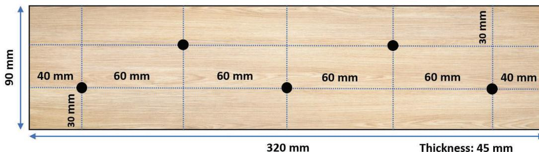
Figure 1. The Layout of nail withdrawal specimens. Black dots represent the nail driving locations.
