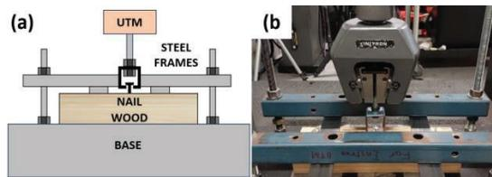
Figure 2. (a) The schematic layout of the NWC test and (b) the actual test layout using metal frames.
