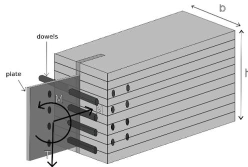
Figure 1. Dowel-type assembly
