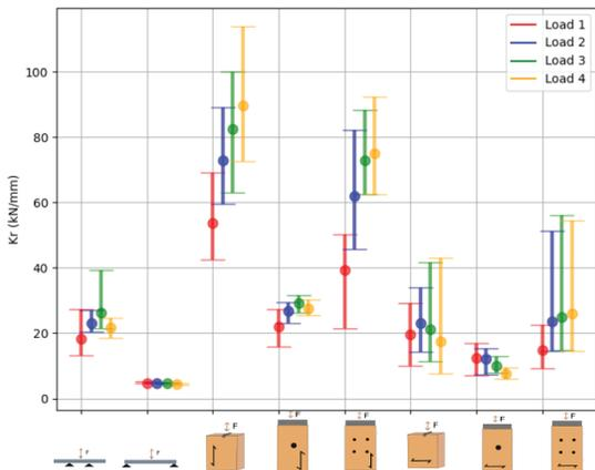
Figure 9. Max., mean and min. of the loading stiffness in the elastic domain and in the plastic domain for all tests configurations.
