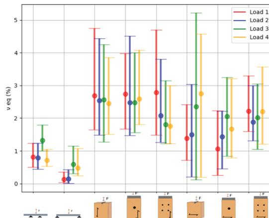
Figure 12. Max., mean and min. of the equivalent viscous damping coefficient for all configurations.
