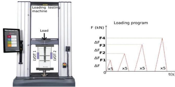
Figure 4. Tests set-up (left) and loading protocol (right).
