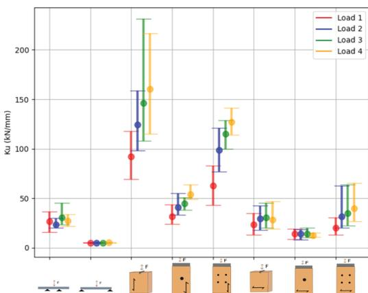
Figure 10. Max., mean and min. of the unloading stiffness in the elastic, and in the plastic domain for all configurations
