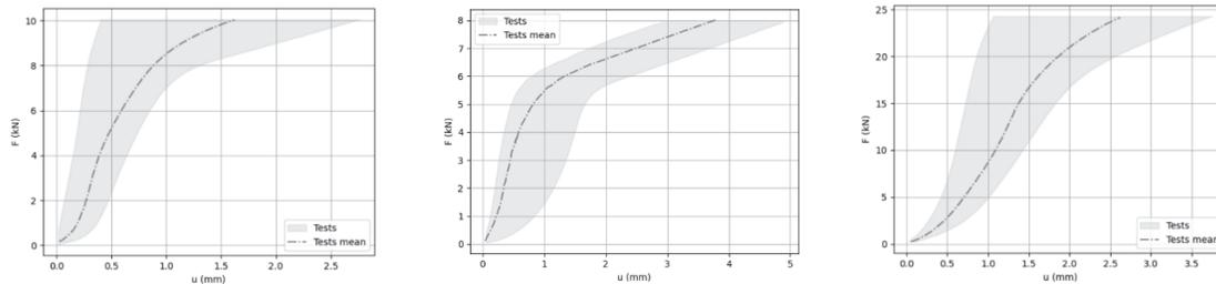
Figure 8. Perpendicular to the grain envelopes: for embedding tests (left), one-dowel assembly tests (middle) and four-dowel assembly tests (right).
