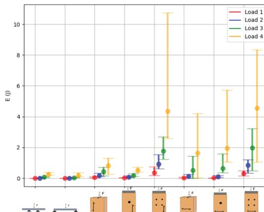
Figure 11. Max., mean and min. of the energy dissipation in the elastic and plastic domain for all configurations.
