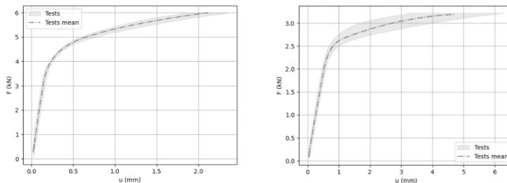
Figure 6. Envelope curves of the dowel tests, of three-point bending test on 5 cm dowel span (left) and 8 cm dowel span (right).
