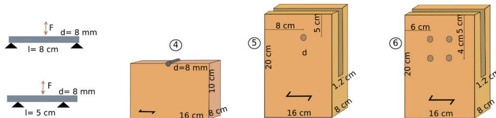
Figure 3. Dimensions of specimens for tests perpendicular to the grain.
