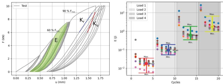
Figure 5. Parameters measured in the force-displacement response (left), representation of the variation of a parameter on the four last cycles at each load level and for given group (right).
