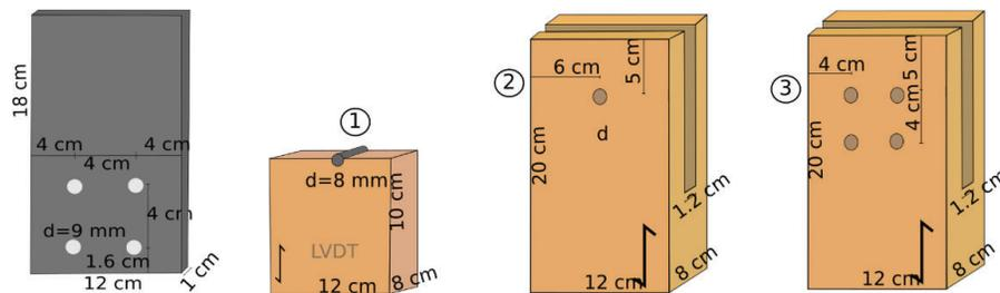
Figure 2. Dimensions of specimens for tests parallel to the grain.
