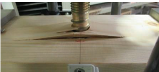
Figure 3. Withdrawal failure with rising up of the surface fibers
