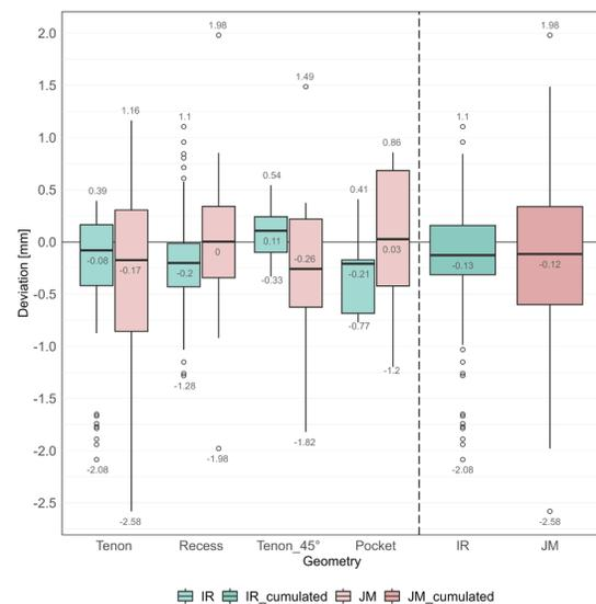
Figure 8: Machining accuracy of the ABB IRB-7600 at BOKU Robot Laboratory and Hundegger k2i at Rubner Holzbau GmbH [9].
