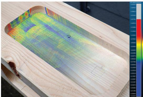
Figure 7: Surface quality inspection visualised by an high-resolution 3D scan [15].
