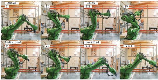
Figure 5: Wrist configurations required to reach the defined positions.
