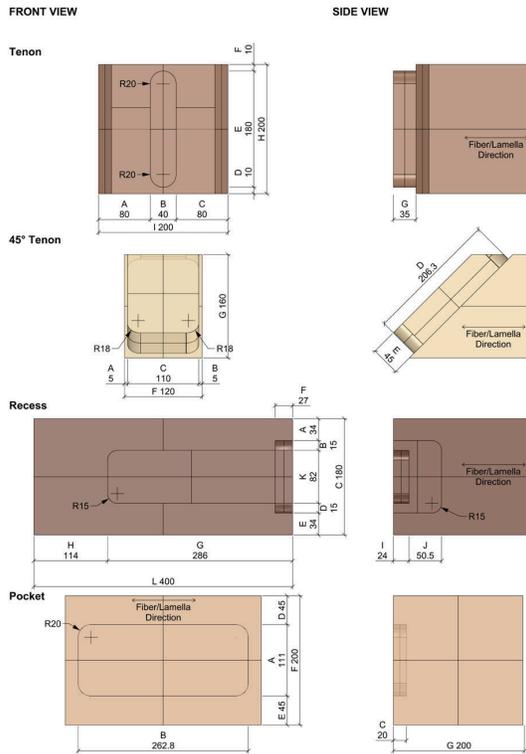
Figure 2: Selected workpiece geometries as subject to the experimental trials. Measured lengths A-L.
