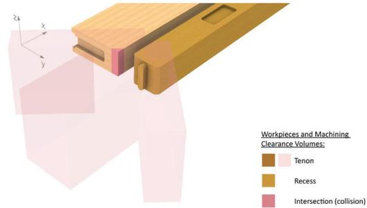
Figure 6: Operating principle of the optimisation model based on penalties for intersecting volumes. An intersection volume of the machining clearance and recess workpiece is shown.
