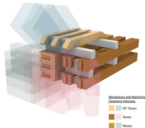
Figure 10: Workpiece stack as optimised by the parameterised model consisting of ten workpieces including their machining clearance volumes.
