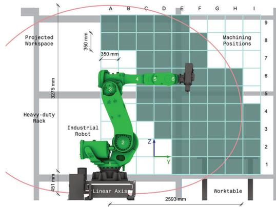
Figure 3: Test setup for accuracy examinations along the workspace.
