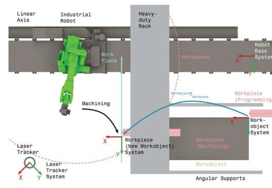
Figure 4: Top view on the trial setup highlighting the coordinate transformation and test setup for accuracy examinations along the workspace.
