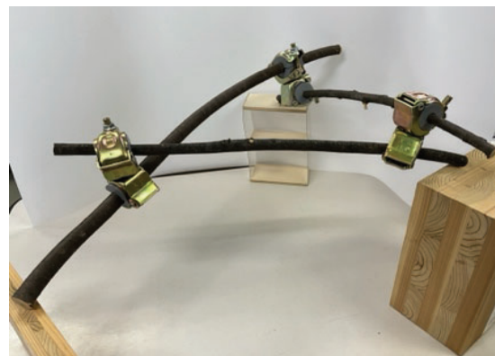
Figure 11. A triangular module with a reciprocal frame structure using the wood A-C.
