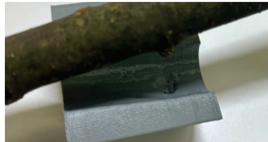
Figure 9. A 3D printed joint that can fit into wood.
