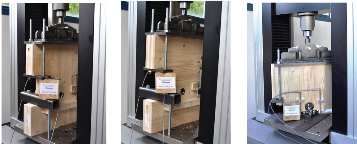
Figure 5. RING60T with vertical (left) or horizontal (centre) outer boards and RING90C (right) FIT test setup
