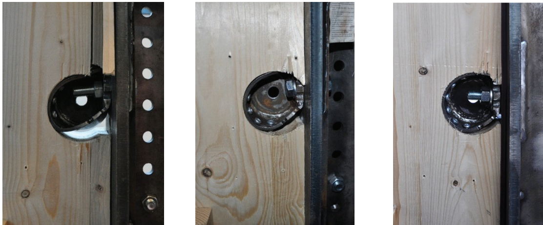
Figure 11. F2/3 failure mode: RING90C-partial pattern (left), RING90C-full pattern (centre- withdrawal) and RING90C with interlayer (right)
