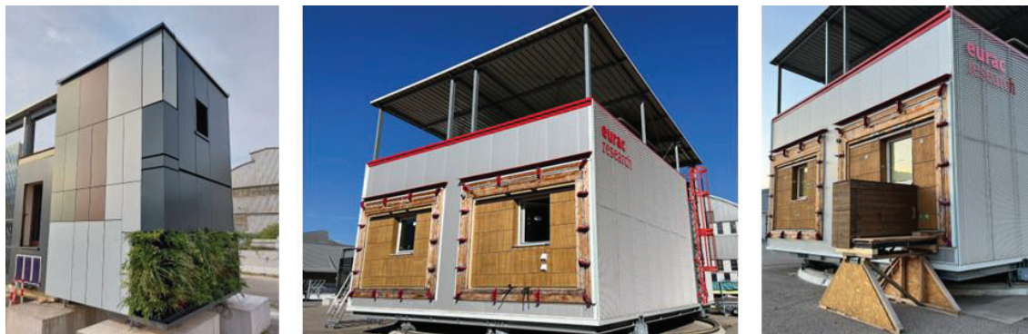
Figure 2. The three full-scale mock-ups, functional mock-up on the left, FSIL with two configurations in the middle and right.
