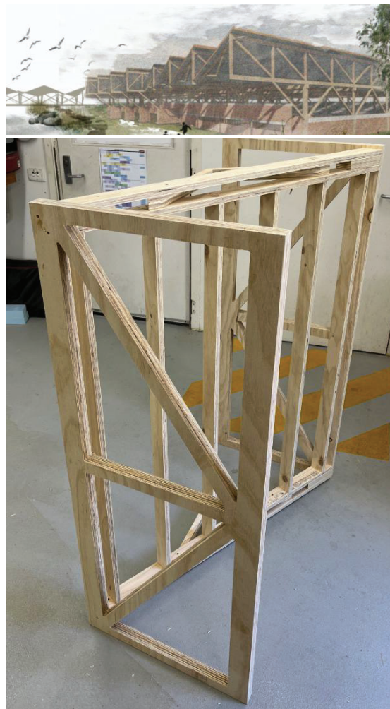
Figure 6. Visualisation of arena roof structure, and prototype of typical timber structural bay at 1:5 scale. Mubashshira Alam
