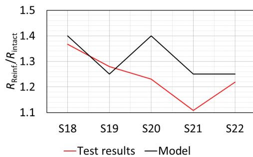
Figure 7. Punching shear test results vs. analytical model.
