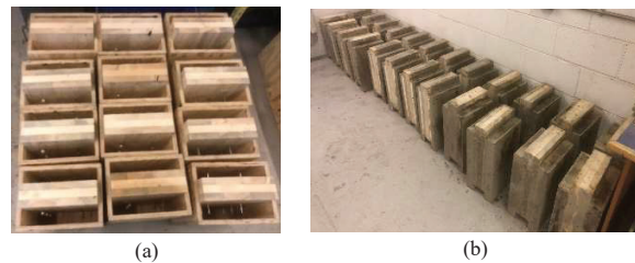
Figure 4: (a) CLT positioned in formwork and (b) experimental TCC specimens
