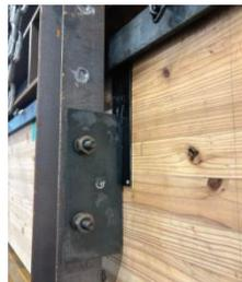
B: Plates for vertical sliding to specimens
