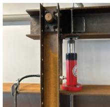
E: An oil jack for adjusting the level of H-shaped steel/C and one-way pin
