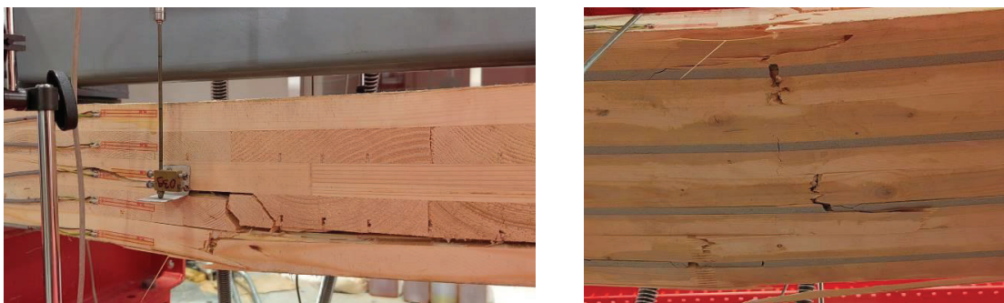
Figure 5. Typical failure mode of the Series C reinforced panels (Specimen C3)
