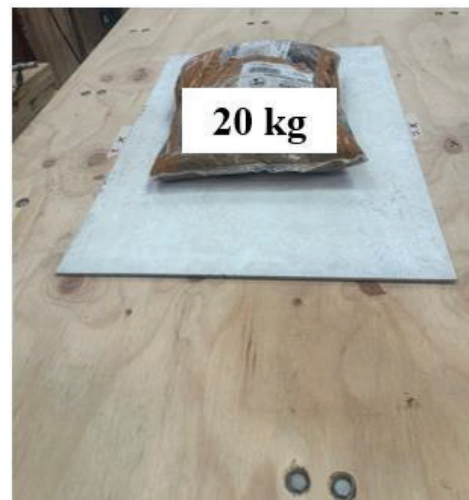
Figure 2: Adding mass (20 kg) on the laboratory timber bridge
