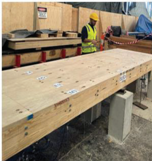
Figure 4: Impact hammer testing on the laboratory timber bridge
