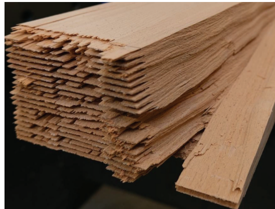
Figure 9: Beam specimen after tension test with high proportion of failure in the finger joints
