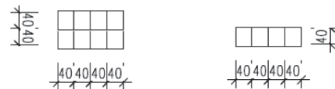
Figure 1: Left: Cross section of a double laminated specimen; right: cross section of a single lamella
