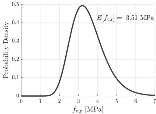
Figure 3: Lognormal distribution of the rolling shear strength, with censored data considered.  $E$  is the expected value.
