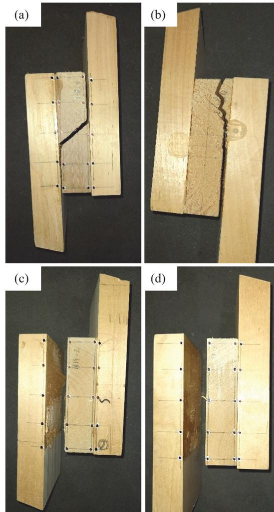
Figure 2: Different failure modes from the rolling shear tests showing failures in the rolling shear specimen (a & b) and along the bond-surface (c & d). Images from Jungerstam 2023 [12].
