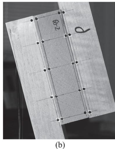
Figure 1: (a) Schematic of rolling shear test setup and dimensions (mm) and, (b) black and white point tracking points on the rolling shear specimen and load transfer plates.
