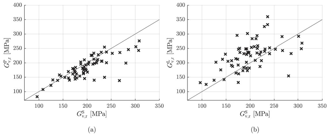
Figure 4: Comparison of the shear modulus determined based on (a) point tracking points on the rolling shear specimen  $G_{v,r}^S$  versus point tracking points on the loading plates  $G_{v,r}^P$  and (b) point tracking points on the rolling shear specimen versus LVDT measurements  $G_{v,r}^L$ .
