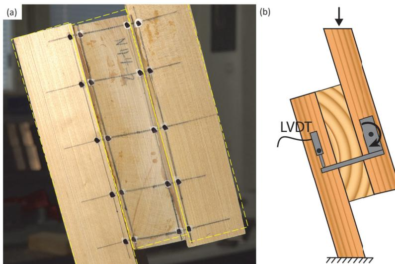
Figure 5: (a) A specimen loaded to  $F = 50$  kN showing the deformed shape along with the initial unloaded shape outlined in yellow dashed lines and (b) The influence of clockwise rotations on the LVDT measurement setup.
