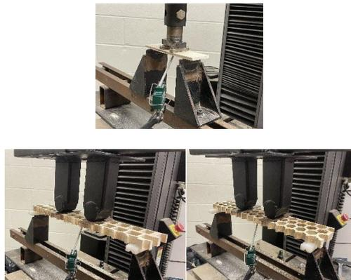
Figure 4. Plywood face specimen (top), the softwood aspen core specimen (bottom left) and honeycomb (bottom right) aspen core specimen under the four-point bending test
