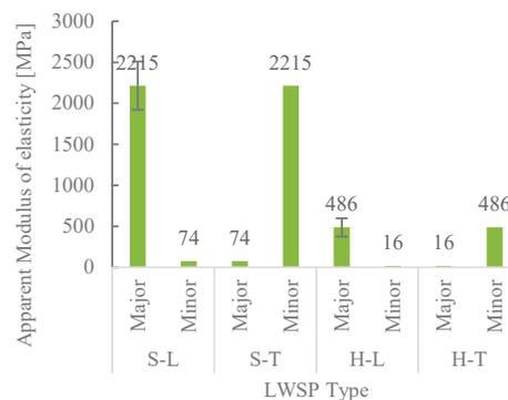
Figure 6. Modulus of elasticity (MPa) of cellular cores
