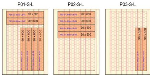
Figure 3. Cutting layouts for LWSP bending specimens from S-L panels
