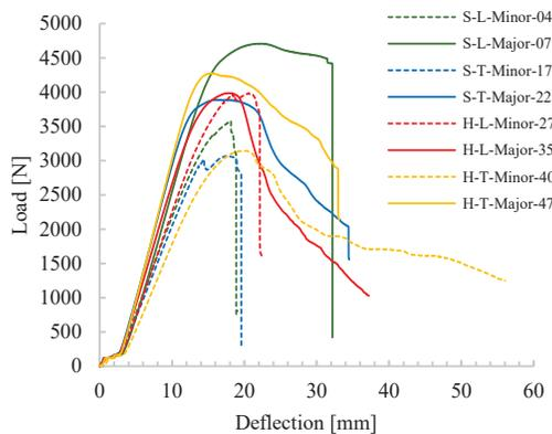
Figure 7. The load-deflection curves of LWSPs
