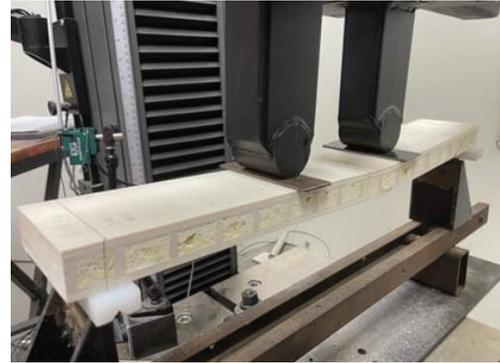
Figure 5. LWSPs bending specimens under the four-point bending test
