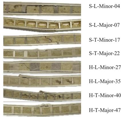
Figure 8. Failure modes of LWSP
