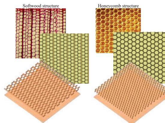
Figure 1. Natural softwood and honeycomb cellular structures
