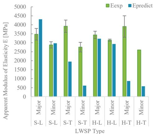
Figure 10. Comparison between theoretically predicted and experimentally tested apparent modulus of elasticity
