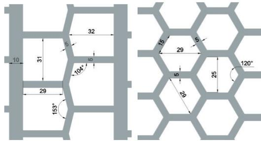
Figure 2. Geometry and dimensions of softwood (left) and honeycomb (right) cellular structure
