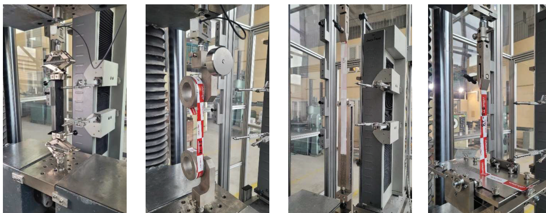
Figure 3 - From left to right: EN 12311-1, EN ISO 29864 method B, ISO 29862 at 180° and 90°
