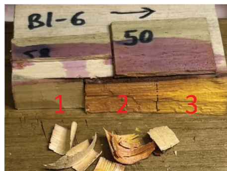
Figure 2. Sample showing check surfaces split for shavings collection and chemical analysis.
