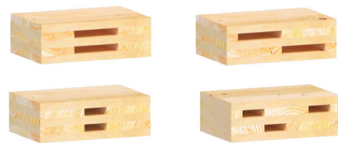
Figure 1. Examples of airgap configurations in CLT panels.
