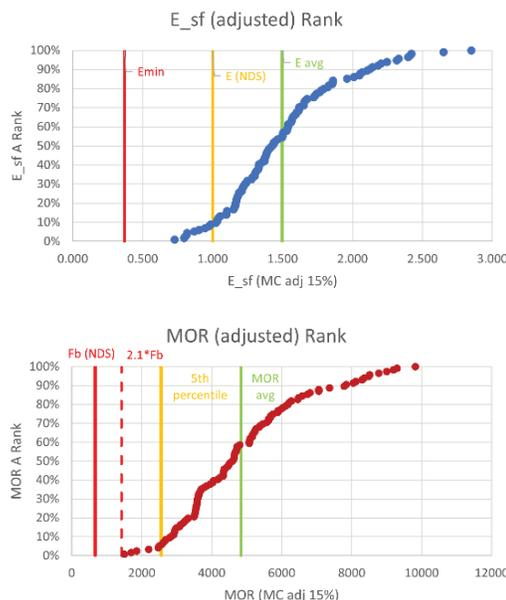
Figure 15. Graphs show relative ranking of shear-free elastic modulus ( $E_{sf}$ ) values (top) and modulus of rupture (bottom) [11]
