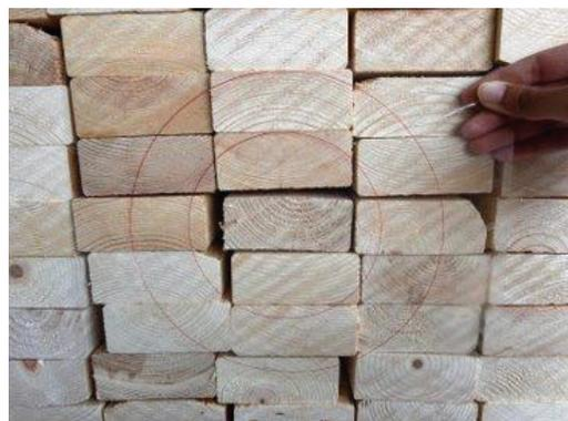
Figure 7. Circle template used to select lumber based on ring curvature in the cross sections [11]
