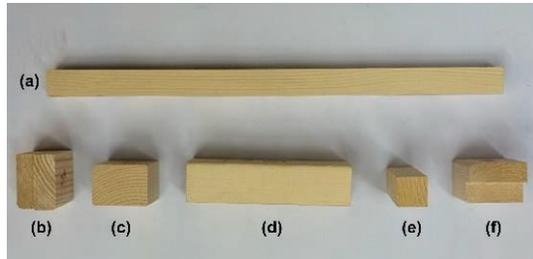
Figure 9. Small clear specimens from top view: (a) static bending; (b) block shear; (c) compression perpendicular (standard); (d) compression perpendicular (modified); (e) compression parallel; (f) block shear (rotated) [13]
