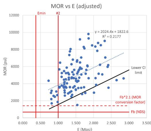
Figure 16. Visual comparison between experimental data and NDS values for first set of bending tests [11]
