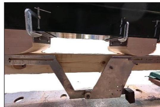
Figure 12. Yoke for measuring deflection in third-point bending [11]
