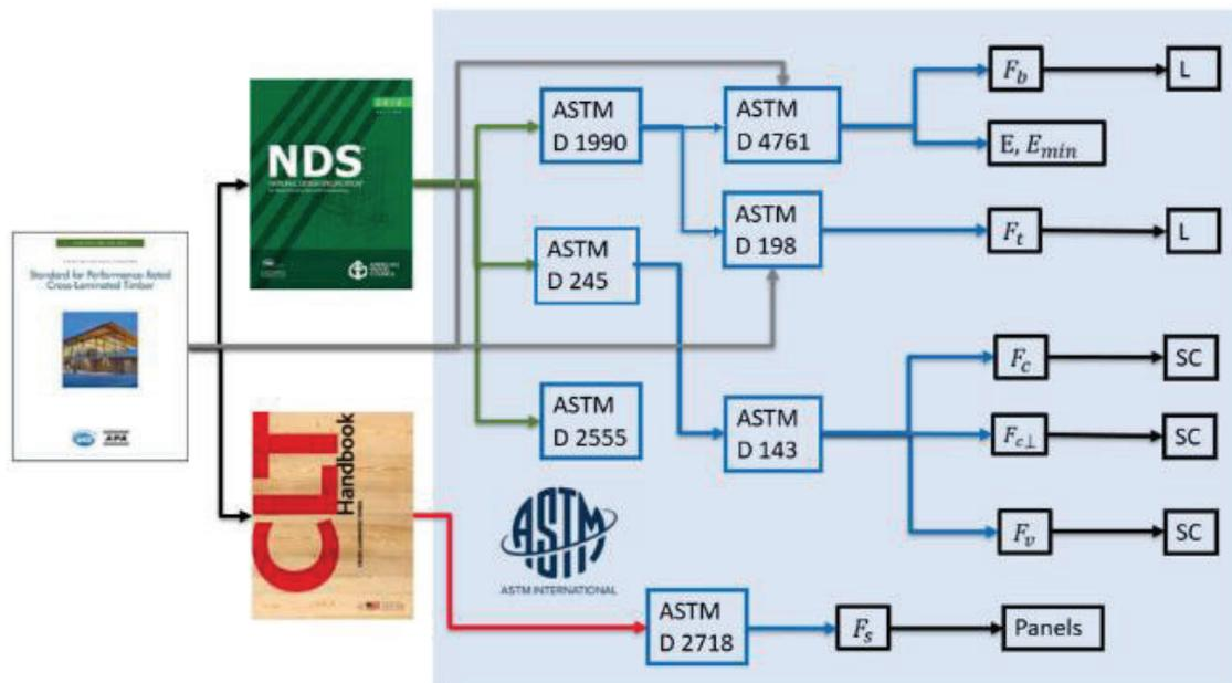
Figure 5. Diagram of references between relevant standards used to select test procedures for each mechanical property [11]
