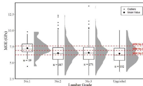
Figure 3. Experimental dynamic modulus of elasticity (MOE) values compared with NDS requirements [4]
