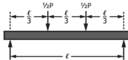
Figure 11. Third-point loading diagram [7]
