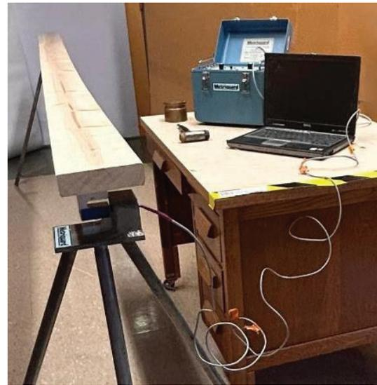
Figure 10. Metriguard set up for dynamic modulus measurement [11]
