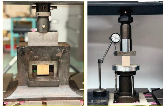
Figure 14. Experimental set up for block shear test (left) and compression perpendicular to grain test (right) [13]
