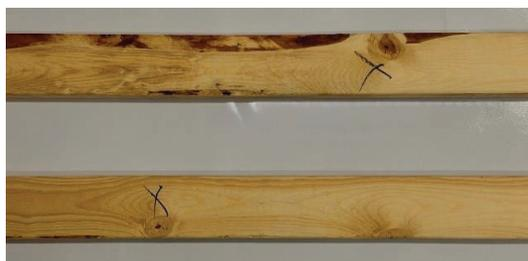
Figure 8. Examples of grade limiting defects [11]
