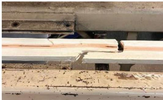
Figure 13. Tension test set-up (top) [14] and close view of example failure (bottom) [11]
