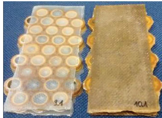
Figure 1. Test specimen (COMBOO with glass / flax fibres) [14]
