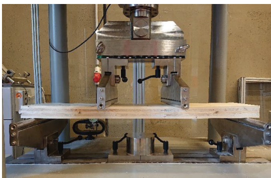
Figure 3. Testing machine with 5 layer CLT (scaled)
