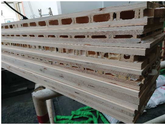
Figure 2. Test specimen CLT / CCLT with different bamboo diameter
