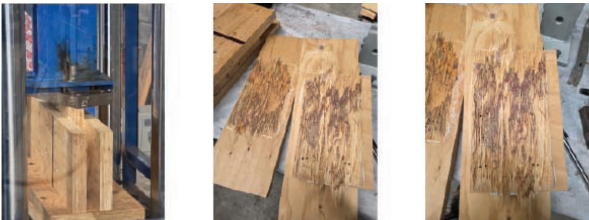
Fig 6: Test C: Left image, failure within panel 3C within the timber fibres. Middle image, successful glue connection achieved without fixings. Right image, complete glue connection and failure after 360.7kN of force.
