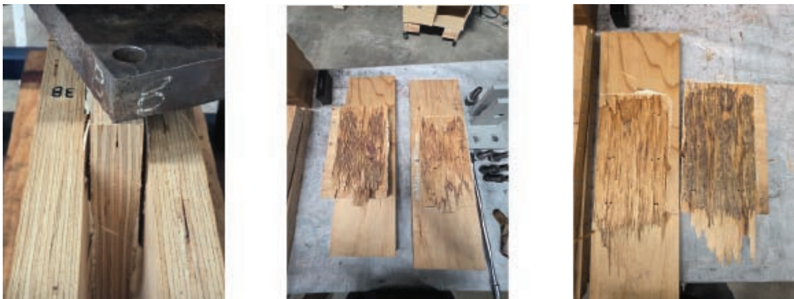
Fig 5: Test B: Left image, failure within both panels 1B and 3B located within the timber fibres. Middle image, pried open specimen showing complete glue connection. Right image, other side of the specimen showing successful glue connection.
