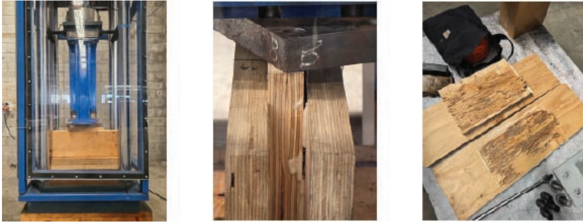
Fig 4: Test A: Left image, Test setup within 1500kN hydraulic press. Middle Image, failure of Panel 1A within the timber fibres. Right image, pried open specimen showing the amount of successful glue connection.
