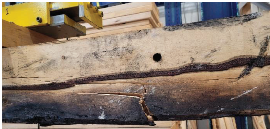
Figure 10: Failure in tension zone of GLT-1, between the loading points
