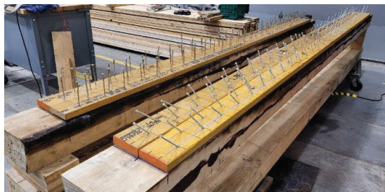
Figure 6: Installation of SK (left) and VGZ (right) screws
