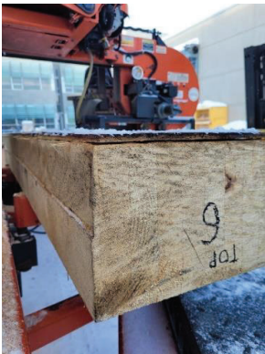
Figure 3: WoodMizer used to reduce the thickness of the char-damaged glulam elements
