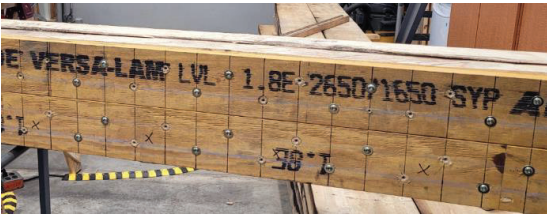
Figure 4: LVL used as reinforcing tension lamination
