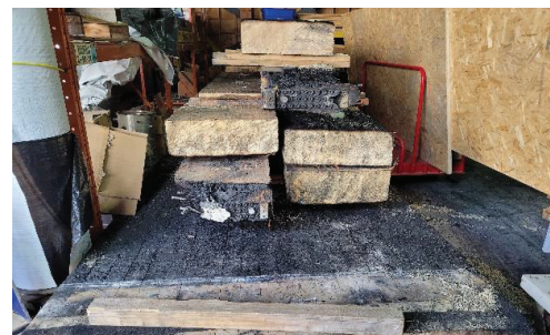
d) Char-damaged elements at FPInnovations
