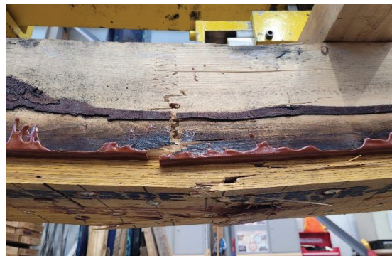
Figure 11: Failure mode observed for the specimen 3-Glue
