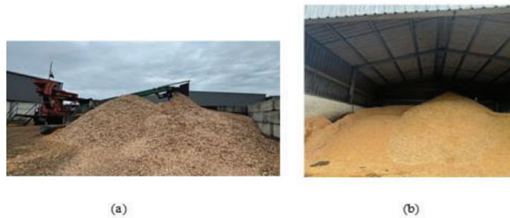
Figure 3: (a) Chipping of timber offcuts for reuse (b) Covered storage of collected wood waste
