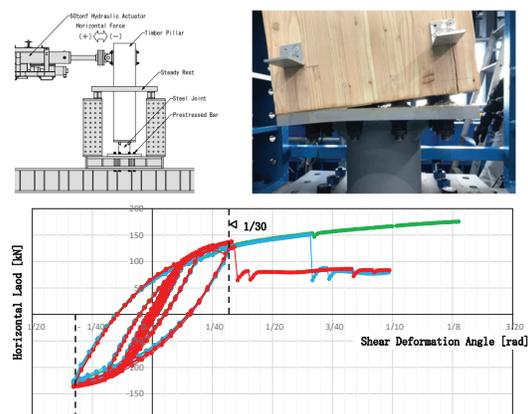
Figure 8: Full-Scale Experimental Results of Timber Column Base
