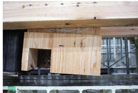
Picture 2: rotation of column-beam joint
