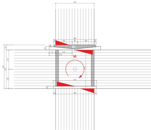
Figure 13: Conceptual Illustration of Rotational Stiffness of the Nuki Joint
