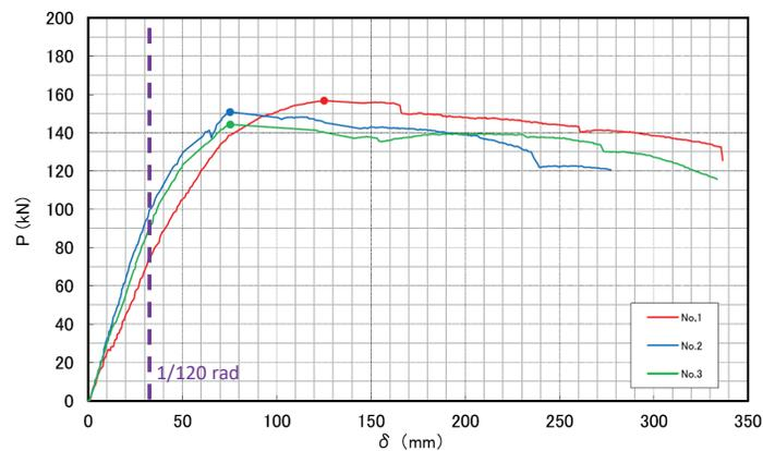
Figure 15:  $P-\delta$  curve of each specimen
