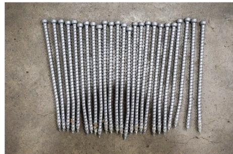
Picture 6: deformation of the wood-wood screws
