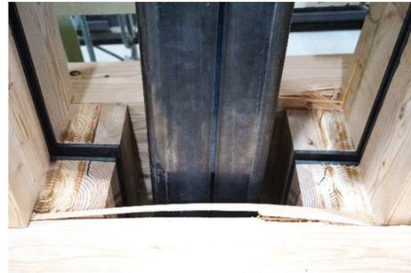
Picture 4: cleavage of the beam
