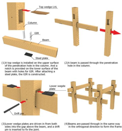
Figure 12: Configuration of the 'Nuki Joint' for Enhanced Rotational Stiffness
