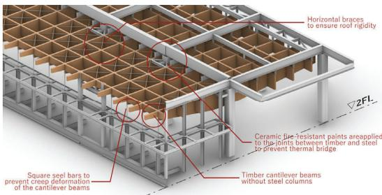
Figure 5: Structural system of the cantilever roof
