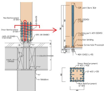
Figure 7: Detailed Drawings of Timber Column Base Joint
