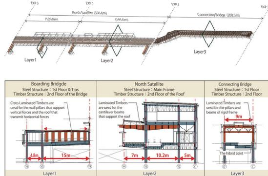
Figure 2: Three layers of the timber-steel hybrid structure
