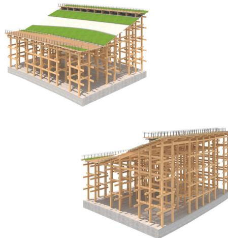
Figure 11: Model of the Two-Way Frame Timber Structure
