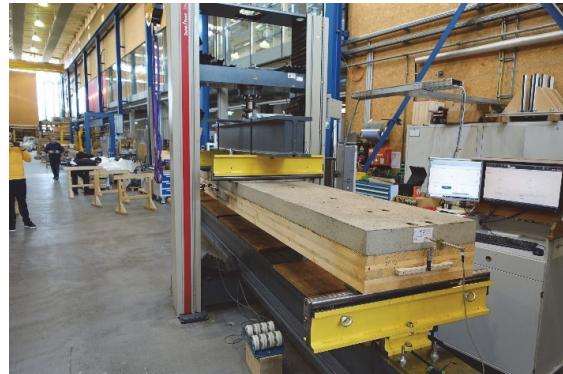
Figure 4. Timber-concrete composite structural floor
