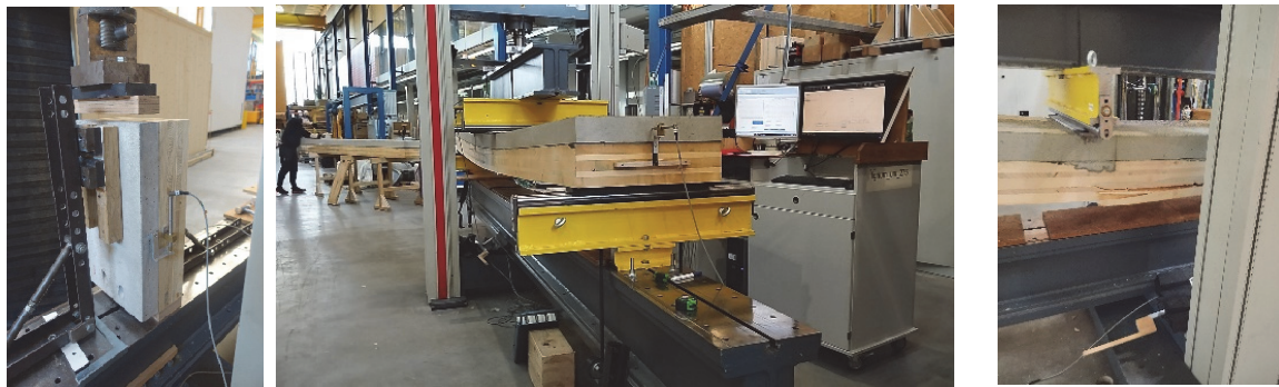
Figure 7. Push-out shear and 4-point bending tests on timber-concrete composite structural flooring system.
