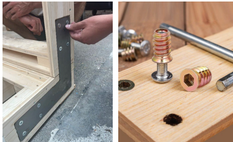
Figure 4. Metal L-shape brackets connected with removable screws
