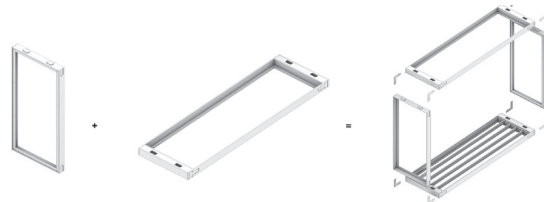
Figure 6. Minimum two walls and two horizontal components are needed to create a segment.
