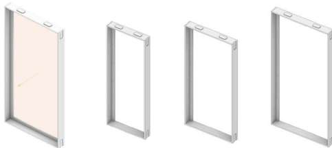
Figure 5. All components use a rectangular reference surface as a reference (left). From the reference surface many variants can be modelled (right).
