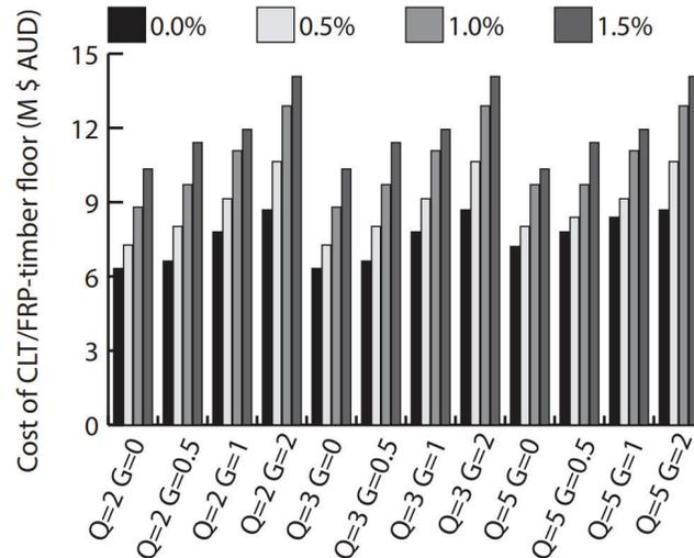
**Figure 5. Cost comparison of CLT volume cost compared to FRP-timber alternatives for the volume reduction scenario (Case 1).**
