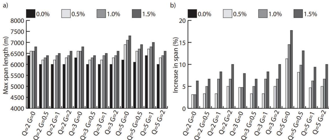
Figure 6. Maximum span of slabs for different load scenarios and reinforcement ratios, and b) span increase for different load scenarios and reinforcement ratios.
