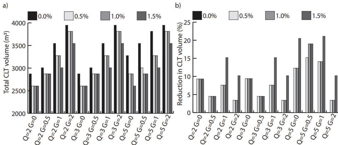
Figure 4. a) CLT volume in slabs for different load scenarios and reinforcement ratios, and b) volume of CLT reduction for different load scenarios and area reinforcement ratios.
