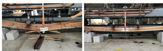
Figure 10 The failure modes of DLT-60 and DLT-90
