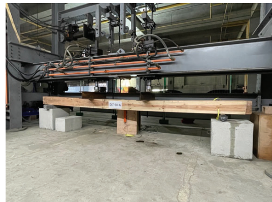
Figure 3 Four Point Bending Test
