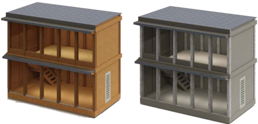
Figure 10 Simulation of RC–timber house and RC house
