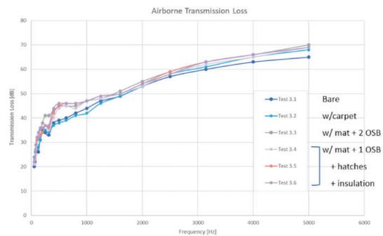
Figure 4. Airborne Transmission Loss Levels Across Test Frequencies
