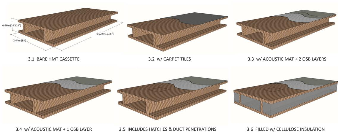
Figure 3. Tested Hollow Massive Timber (HMT) Floor Assemblies
