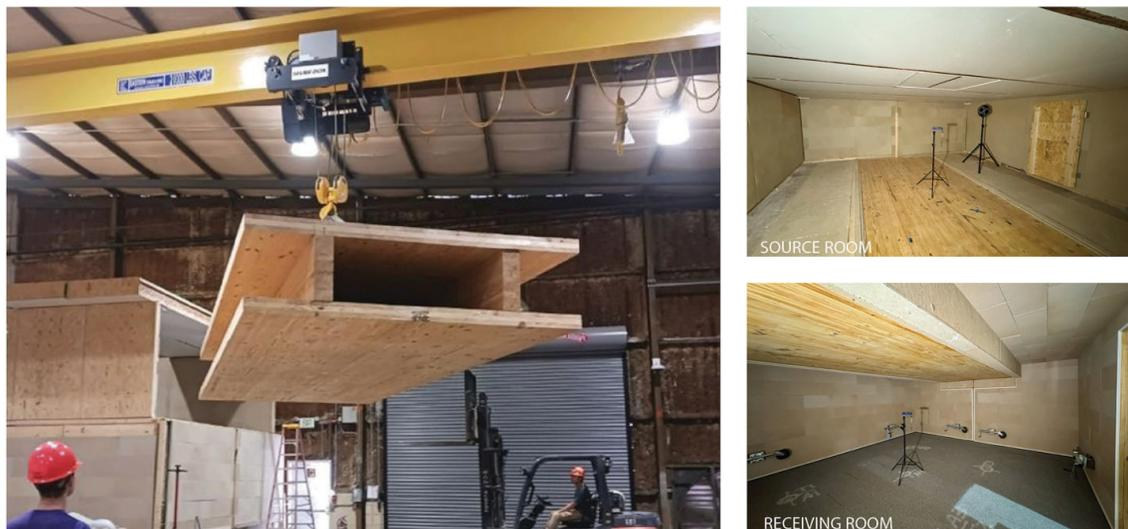
Figure 2. Photographs of Bare HMT Floor Assembly Before and After Installation within Acoustic Chamber
