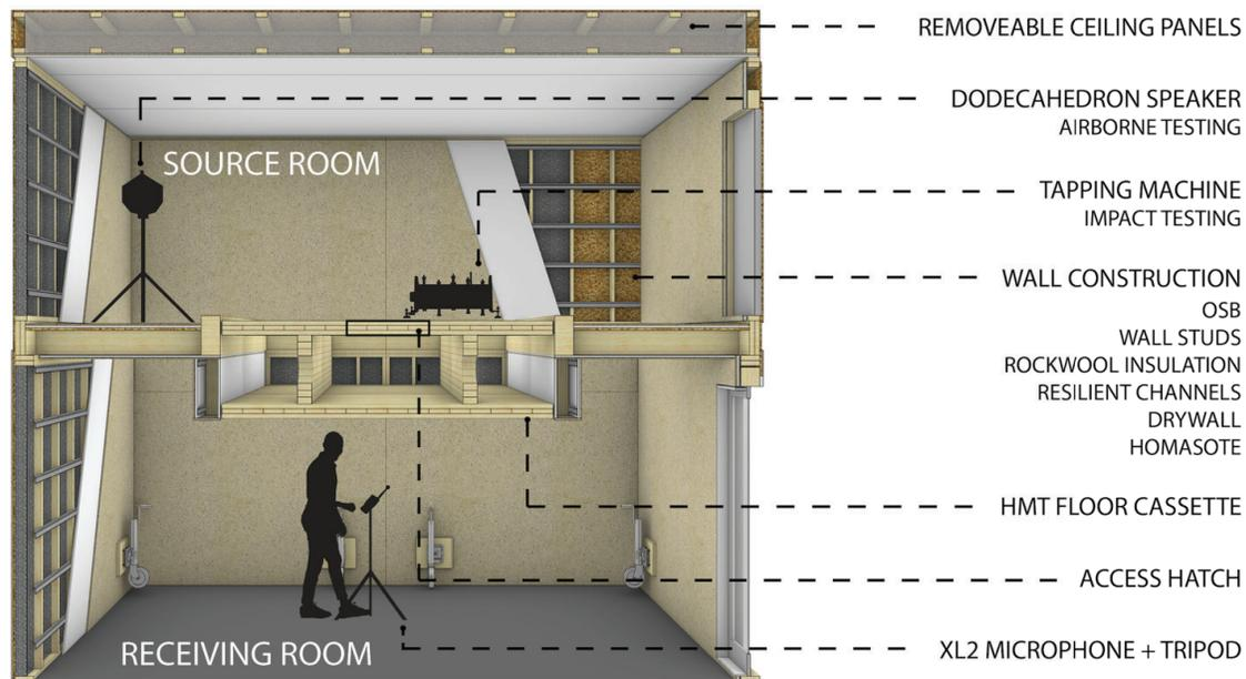
Figure 1. Illustration of Acoustic Chamber and Test Set-up
