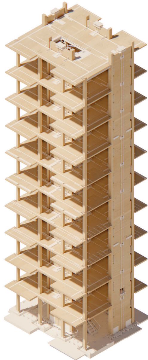
Figure 1. Model of ten-story shake-table test specimen with mass timber structural members and steel connections shown. Positioning and layout of floor diaphragm steel connections varies by mass timber material type used at each level.
