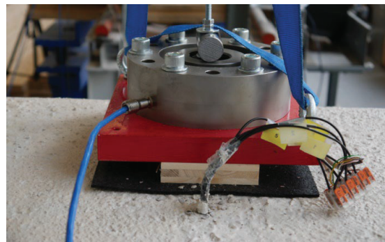
Figure 8. Load cell to qualitatively measure the uplift force curve in the notch
