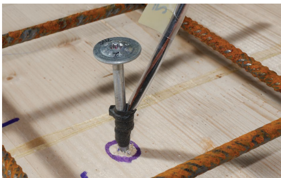
Figure 7. Measuring screws with applied strain gauges in the CLT surface and reinforcement mesh
