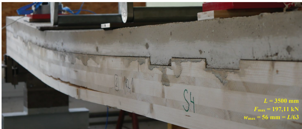
Figure 1. Largely deformed concrete composite test specimen with CLT [6] failed in tension at the bottom lamination
