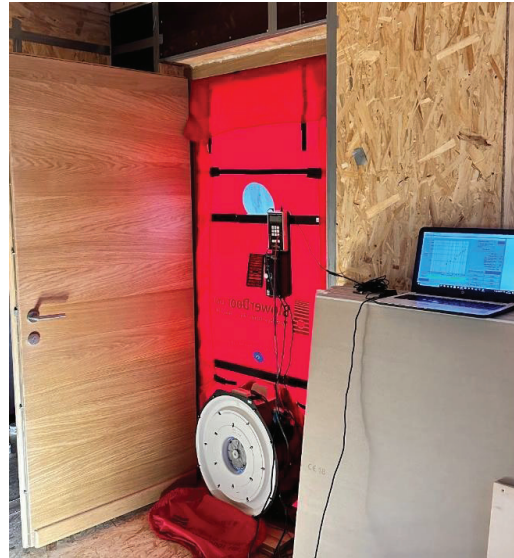
Figure 10 Assembly for blower door test
