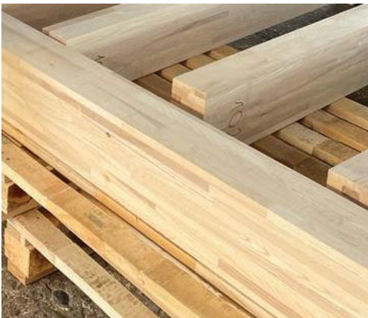
Figure 5 Beams laminated in length, width and thickness
