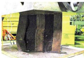
Photo16. A longitudinal compressive force was applied to the specimen in a saturated condition
