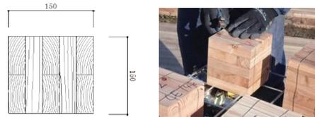
Figure 2. Photo1. Shape of CLT specimens used in exposure tests
