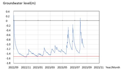
Figure 6. Changes in groundwater level from one to two years after exposure (Subtropical zone)
