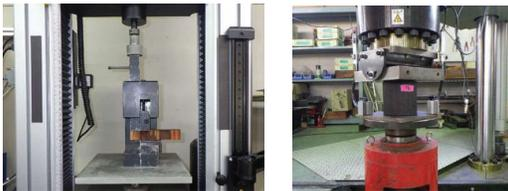
Photos 8&9. block shear test (Left)
