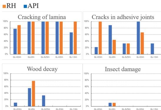
Figure 7. (Number of specimens in which each degradation item occurred)/(Total number of specimens) [%] Subarctic
