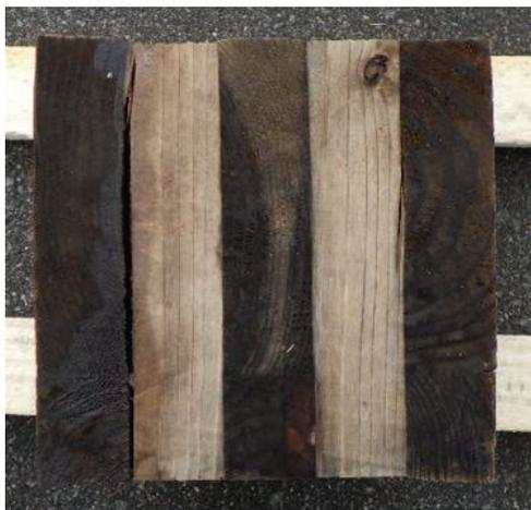
Photo14. Cracking at the adhesive layer Subarctic × API × GL-0.5m
