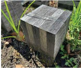
Photo 4. CLT test specimen after two years of exposure (subtropical zone)
