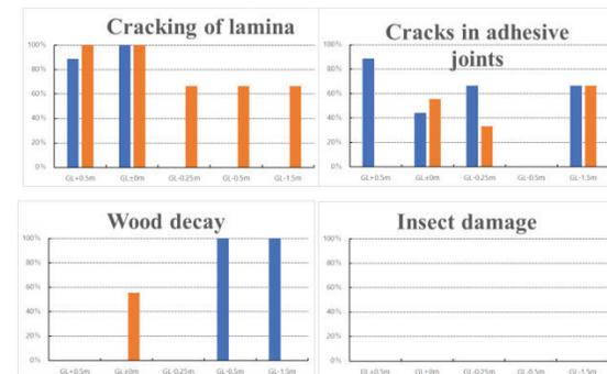
Figure 8. (Number of specimens in which each degradation item occurred)/(Total number of specimens) [%] Temperate
