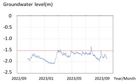
Figure 5 : Changes in groundwater level from one to two years after exposure(Subarctic zone)
