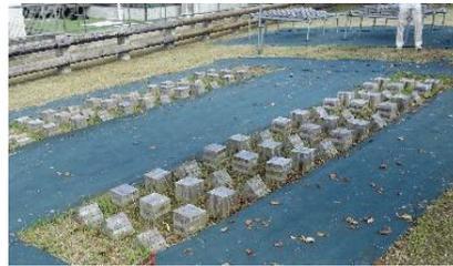
Photo2. Ground installation conditions (Buried the test piece under the blue sheet)
