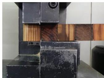
Photo15. Block Shear Test in Progress
