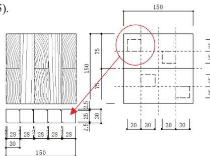
Figure 10. Drawing of specimens for block shear test
