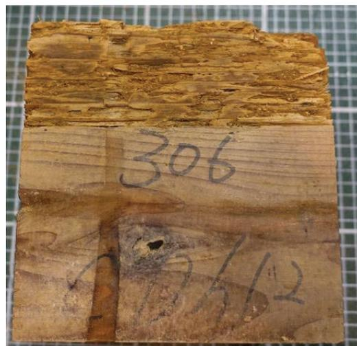
Photo 11. Surface decay (Temperate × APT × GL-0.5m)
