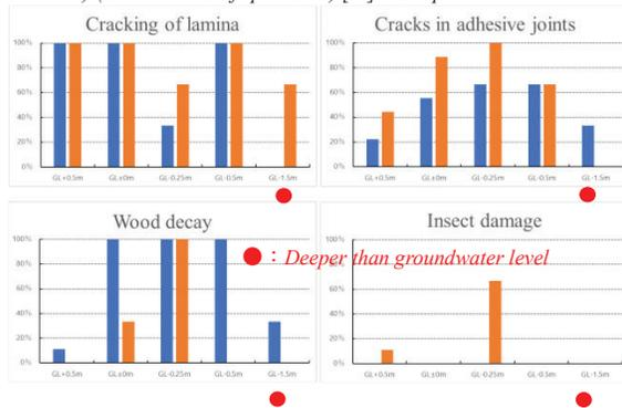
Figure 9. (Number of specimens in which each degradation item occurred)/(Total number of specimens) [%] Subtropical
