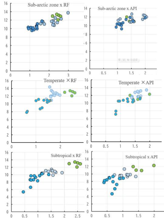
Figure11. Vertical Compressive Strength ●Initial ●1 year ●2 years
