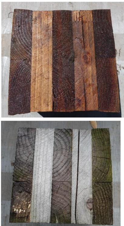
Photo12 &13. Cracking of laminae under the same conditions in subtropical × API Top : GL-0.1m Bottom : GL+0.5m
