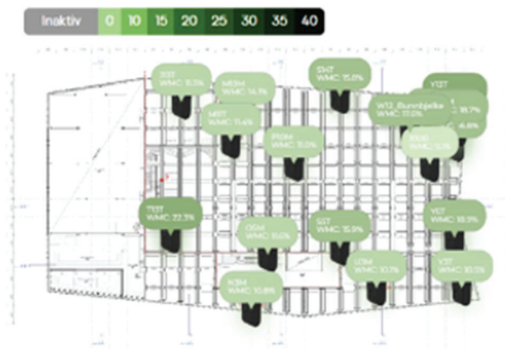
Figure 13: distribution of moisture sensors on the blueprint of the roof (extract from cloud service interface).
