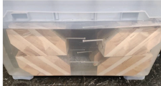
Figure 15: Heavy weathering test specimens totally immersed in water.
