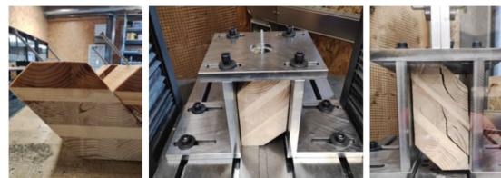
Figure 16: Test specimens (left), system for testing the withdrawal resistance (middle) and specimens with timber failure (right).
