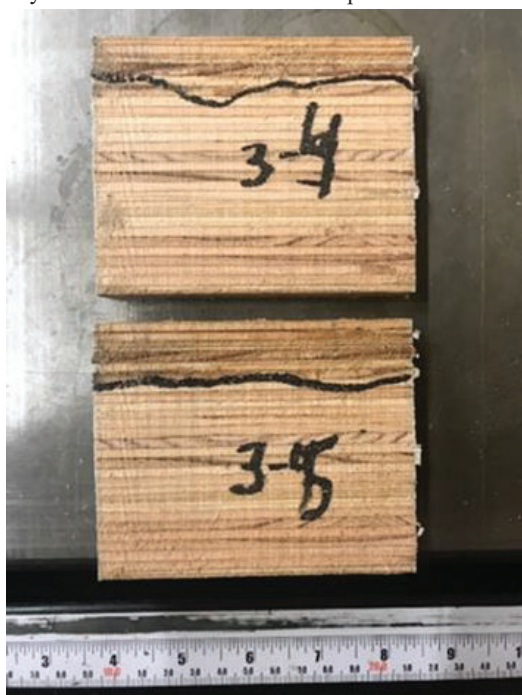
Figure 5. Cross cuts of an MPP panel showing moisture intrusion (darkened area above the marker) after 7 days of wetting.
