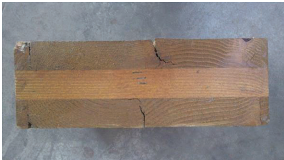
Figure 2. Example of a Douglas-fir CLT panel section exposed to natural rainfall for 30 days and allowed to dry for 2 years showing checking and delamination.
