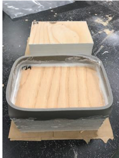
Figure 3 Examples of an MPP block prior to sealing and one sealed with the water well.
